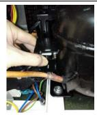
when refrigerant is totally released, remove insulated cotton from low pressure pipe, then remove high and low pressure pipes with welding gun;
